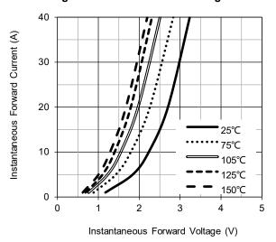
Fig.3 - Typical Forward Voltage Characteristics
