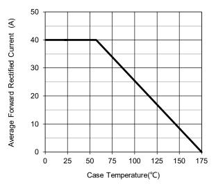
Fig.1 - Forward Current Derating Curve
