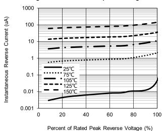
Fig.4 - Typical Reverse Current Characteristics
