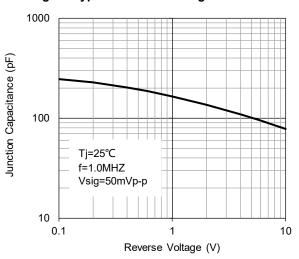
Fig.5 - Typical Junction Capacitance
